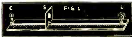
The Bunsen photometer is familiar in every physical laboratory; it operates by balancing the respective intensities of light falling from either side on a translucent spot S.
