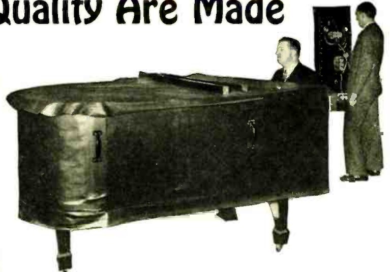
Fig. A A new "power" piano, encased in a sound-proof casket; inside it are specially-arranged microphones to pick up the sound. Through an amplifier, and reproducers, these sounds may be magnified until the pianist can dominate a full orchestra in crescendo. Mr. Cockaday, who is associated with a group of engineers in working out this problem for the Steinways, is seated at the pianoforte.
